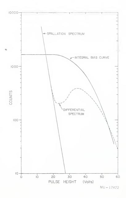
Fig. 12. Method used to extrapolate the integral bias curves to zero bias, i.e., the spallation spectrum was subtracted from the differential spectrum in calculating the integral bias curve.
